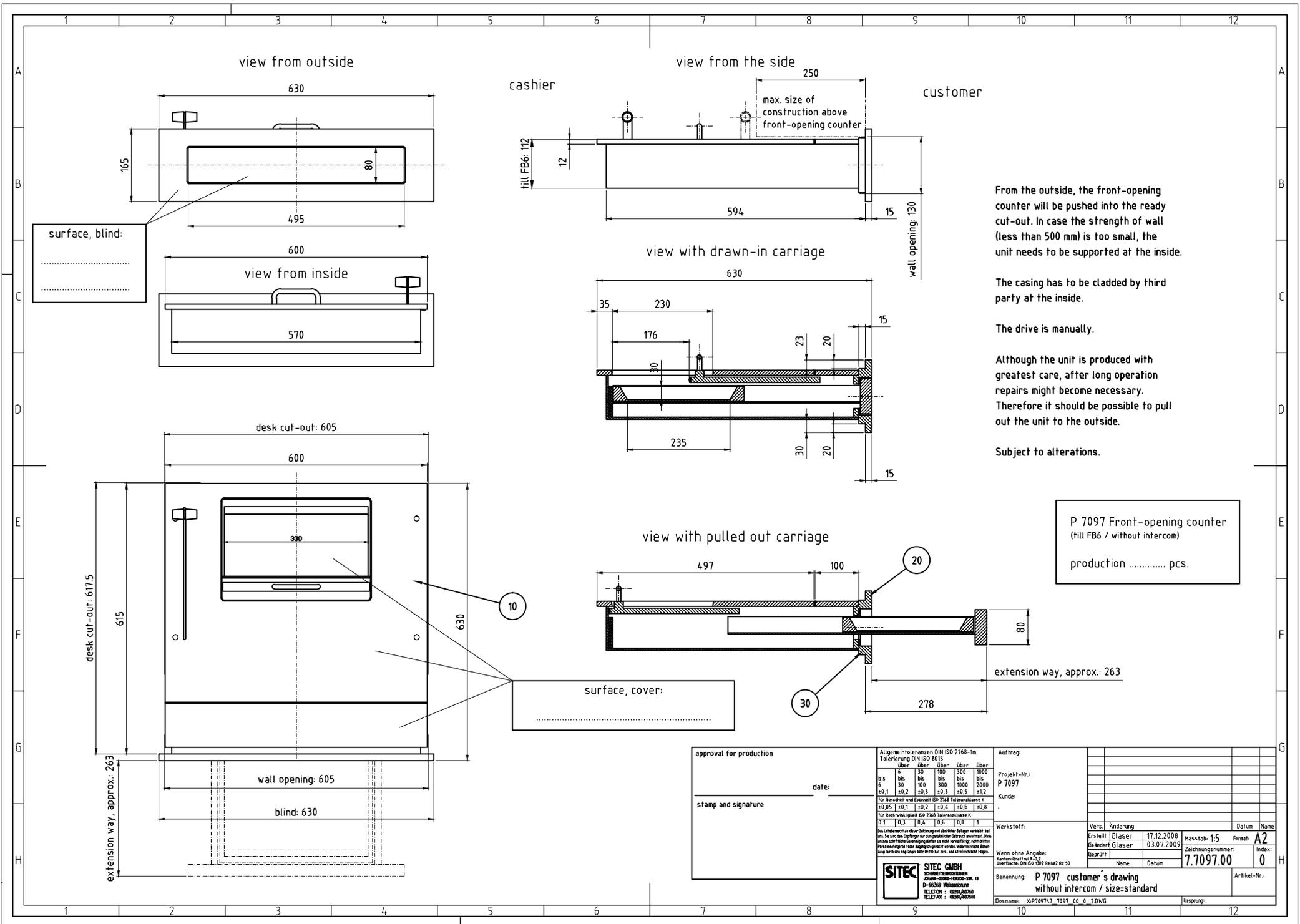
From the outside, the front-opening counter will be pushed into the ready cut-out. In case the strength of wall (less than 500 mm) is too small, the unit needs to be supported at the inside.
